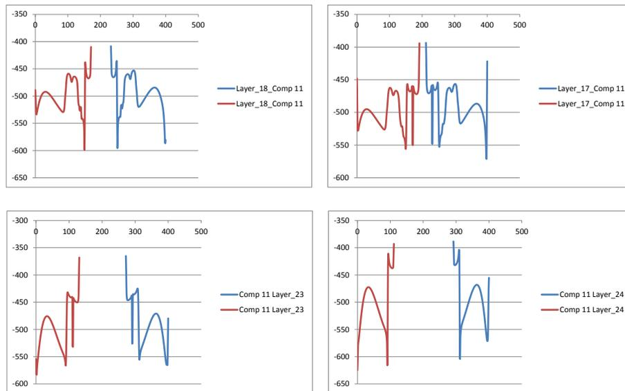
**Figure 12.**  $\sigma_{11}$  stress [MPa] in 0° original plies
