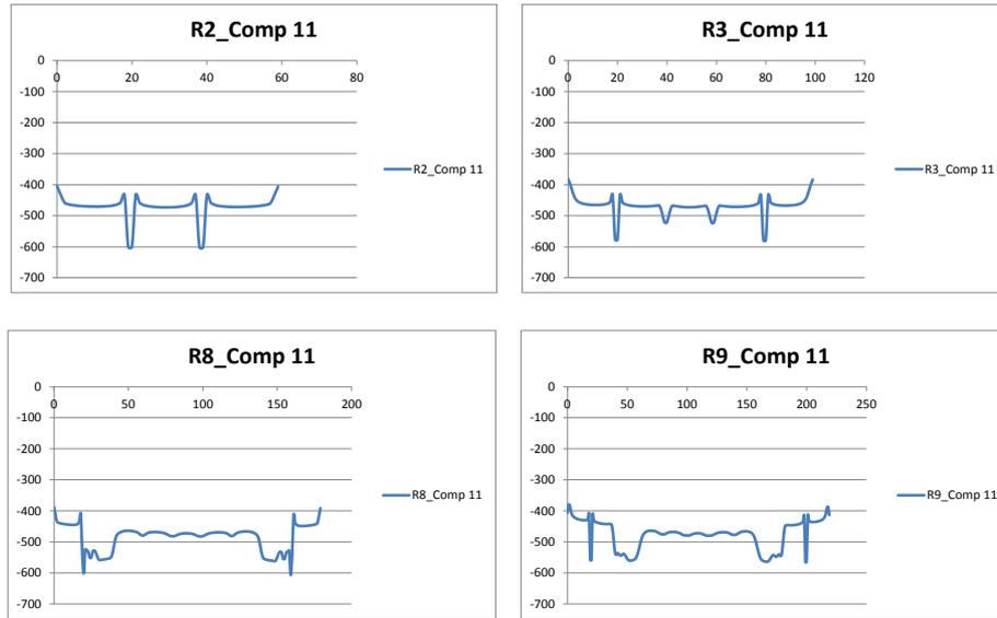
**Figure 11.**  $\sigma_{11}$  stress [MPa] in 0° Repair laminas
