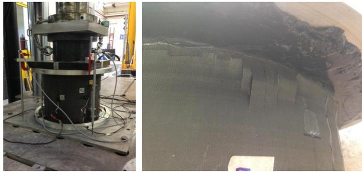
**Figure 15.** Compression Test of undamaged cylinder (reference)
