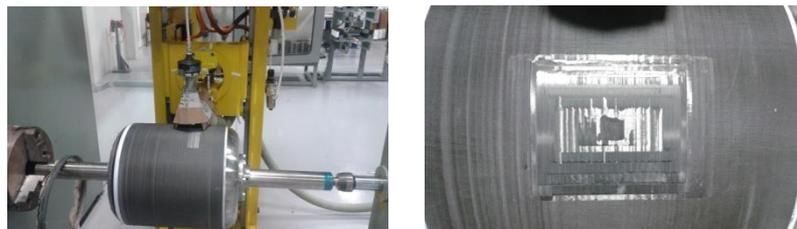
**Figure 8.** Stepped scarfing phase
