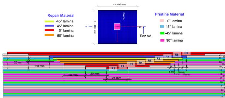
**Figure 5.** Repair scheme
