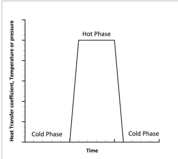
Fig. 3: Thermomechanical load cycle
