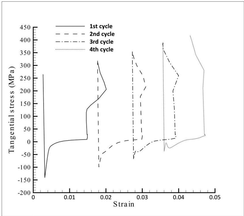
Fig. 6: Tangential Stress vs Total tangential strain - 4 cycles
