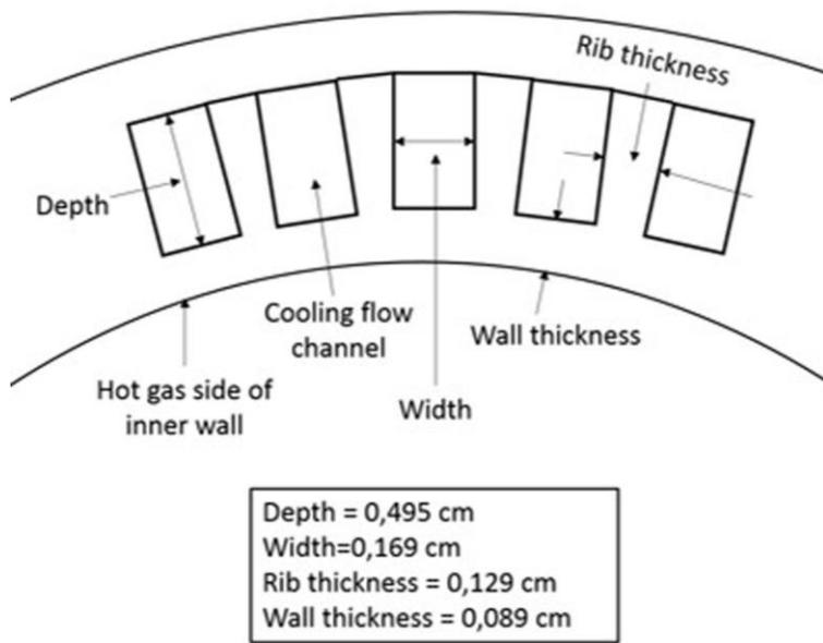
Fig. 2: Cooling channel geometry
