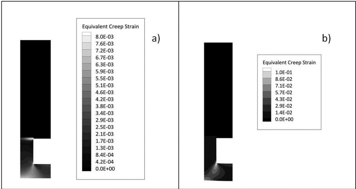
Fig. 7: Equivalent creep strain, (a): creep after 1 second, (b): creep after 240 seconds
