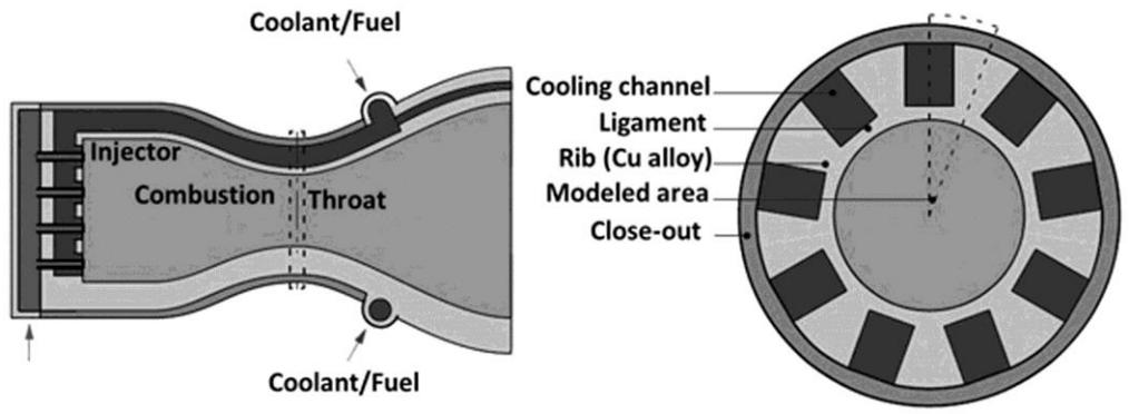
Fig. 1: Scheme of the regenerative liquid rocket engine
