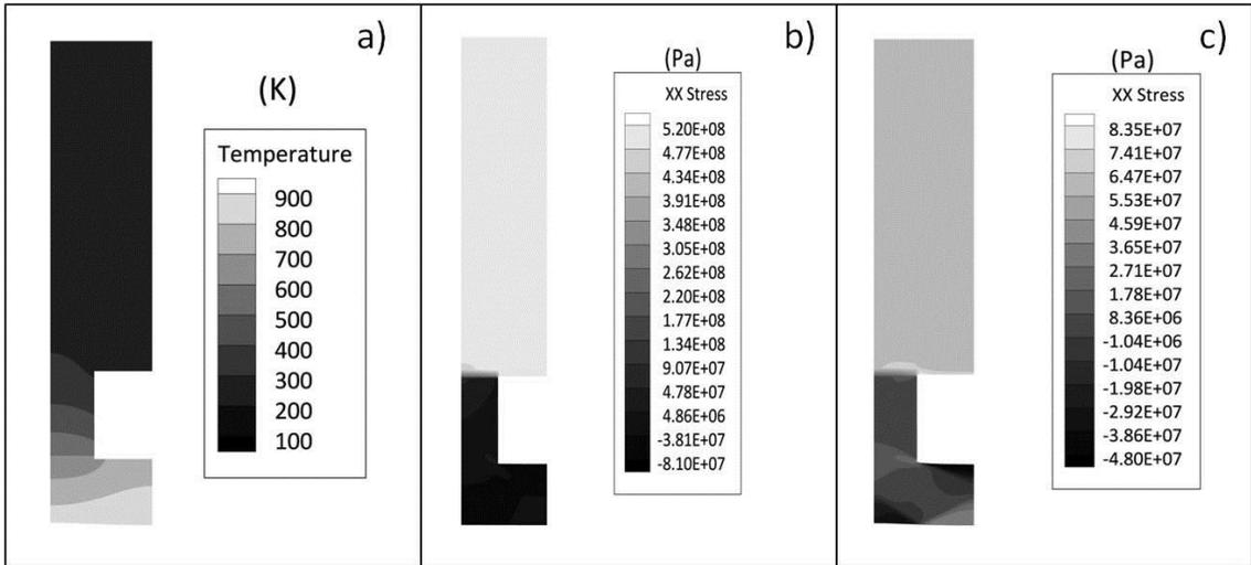
Fig. 5: (a): Temperature contour plot (Hot phase), (b): Hoop tangential stress (creep after 1 second), (c): Tangential stress - creep after 240 seconds
