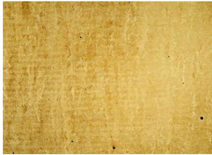
Figure 4-4-a: Micrograph of 50 µm process theme sample showing porosity.
