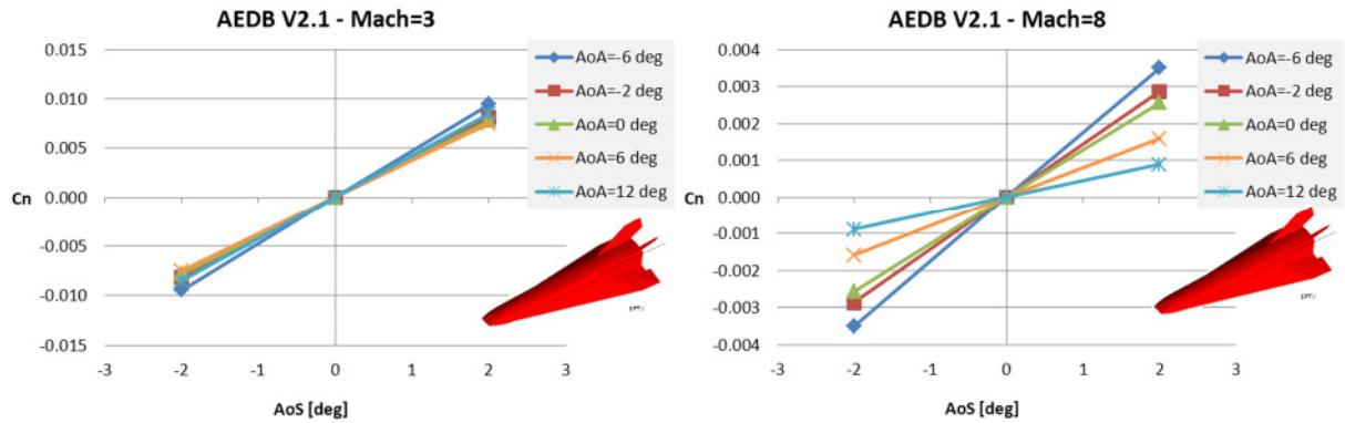
Figure 19.  $C_n$  versus  $AoS$  at different  $AoA$  at  $M=3$  and  $8$ .
