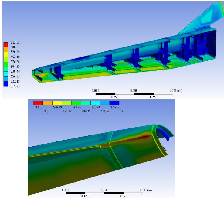
**Figure 22: Temperature distribution on the titanium structure at the peak heating condition for titanium components**
