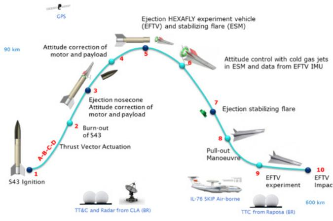
Figure 5: Flight sequence profile
