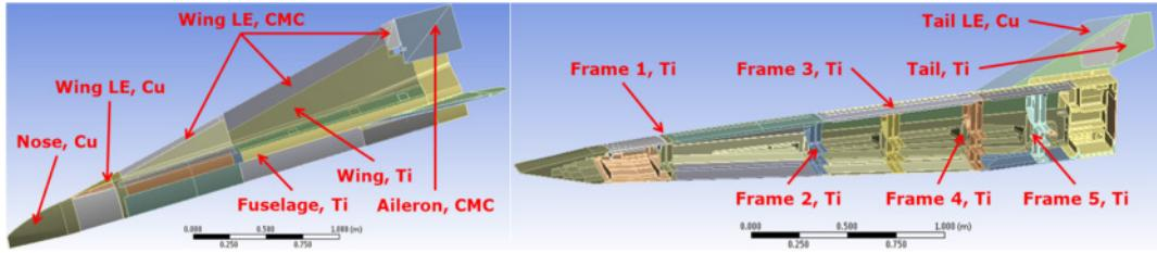
Figure 20: Main structural components of the analysed EFTV
