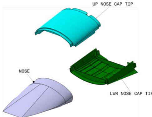
**Figure 13: Nose Cap exploded view**
