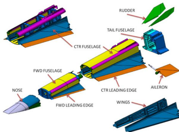
Figure 12. EFTV main components
