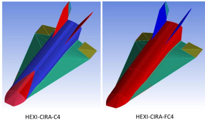
Figure 8: Comparison between CIRA-C4 and CIRA-FC4 aeroshapes.
