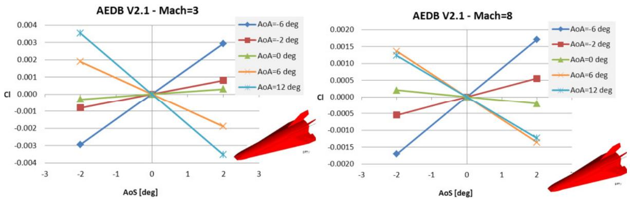
Figure 18.  $C_l$  versus  $AoS$  at different  $AoA$  at  $M_\infty=3$  and 8.
