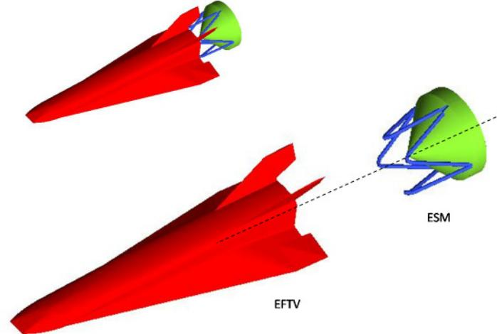
Figure 6: EFTV docked to ESM, EFTV and ESM aeroshapes.
