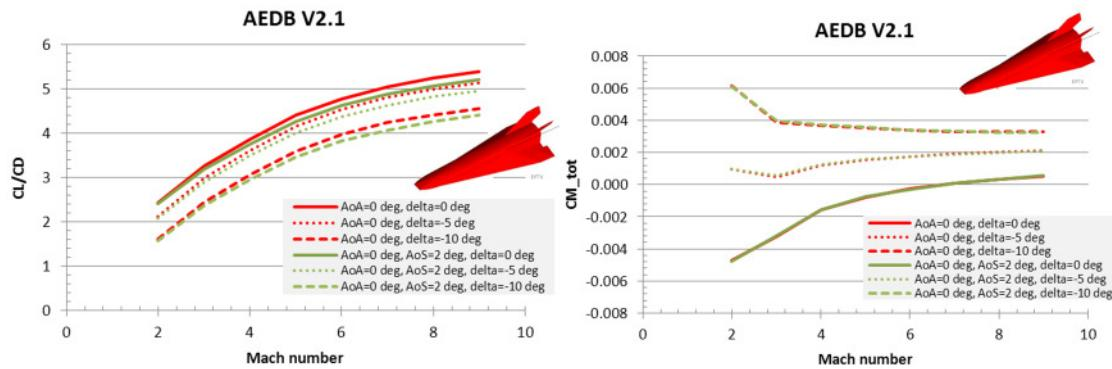
Figure 16. L/D and  $C_m$  vs. Mach number with and without sideslip angle and aileron deflection effects.
