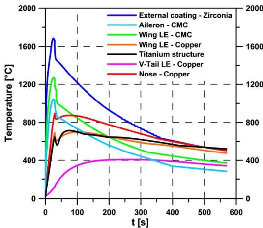
Figure 21: Maximum temperature along the flight profile on the main vehicle components
