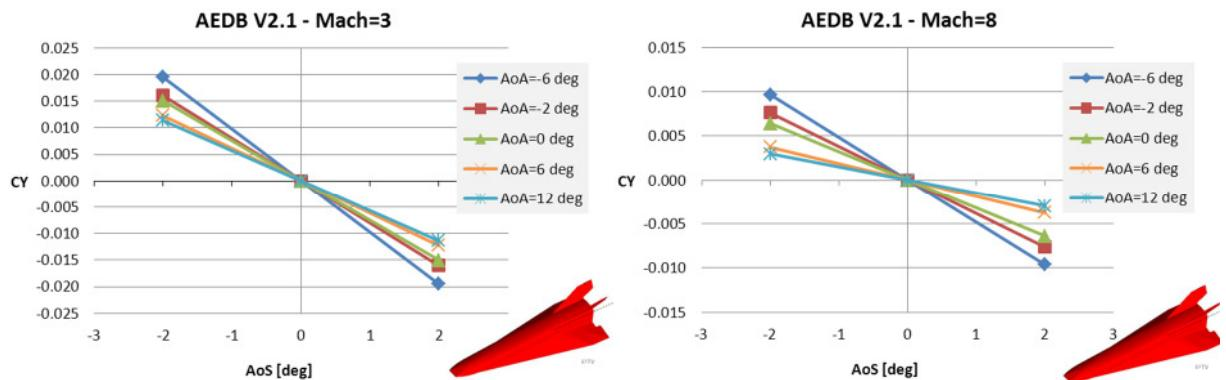
Figure 17.  $C_y$  versus  $AoS$  at different  $AoA$  at  $M_\infty=3$  and 8.
