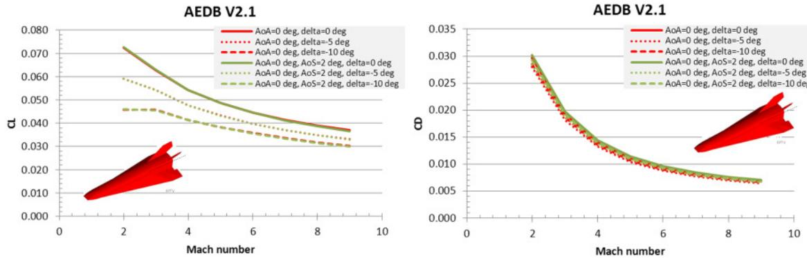
Figure 15.  $C_L$  and  $C_D$  vs. Mach number with and without sideslip angle and aileron deflection effects.
