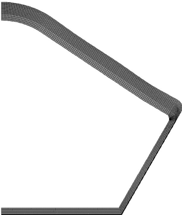
**Fig. 16b.** Initial computational mesh for ID 1336.
